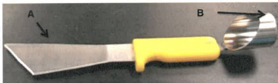
Fig. 1. A typical, commercial lettuce field coring/harvesting knife with A (the cutting blade) and B (the coring ring).
